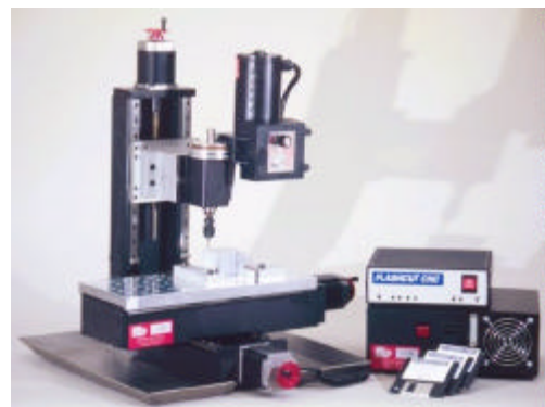
Figure 2. Examples of low-cost 3D CNC milling machines, perfectly suited for RP applications. (sources Delft Spline Systems - left, and Minitech - right).
